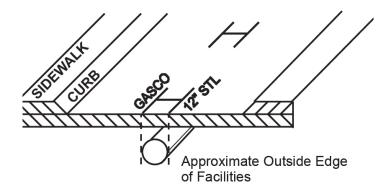
These examples indicate an operator's 12 in. facility. When a facility can be located or toned separately from other facilities of the same type, it is marked as a single facility.<sup>62/</sup>
