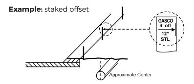
**4.** An operator's identifier (name, abbreviation, or initials) is placed at the beginning and at the end of the proposed work. In addition, subsequent operators using the same color mark their company identifier at all points where their facility crosses another operator's facility using the same color. Reduce the separation of excavation marks to a length that can reasonably be seen by the operator's locators when the terrain at an excavation site warrants.
