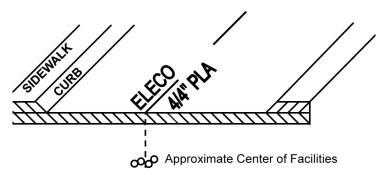
**C.** Conduit Marking: Used for any locatable facility being carried inside conduits or ducts. The marks indicating the outer extremities denote the actual located edges of the facilities being represented.
