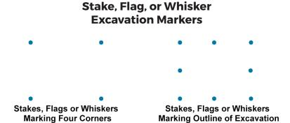
Delineate the proposed area of excavation using stakes, flags, or whiskers instead of spray paint to mark radius or arcs; the four corners of the project; or when outlining the excavation project. Limit the interval spacing to approximately 4 ft to 50 ft. Reduce the separation of excavation marks to a length that can reasonably be seen by the operator's locators when the terrain at an excavation site warrants.
