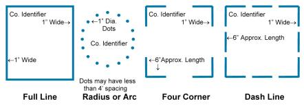
Delineate in white paint the proposed area of excavation using a continuous line, dots marking the radius or arcs, dashes marking the four corners of the project, or dashes outlining the excavation project. Limit the size of each dash to approximately 6 in. to 12 in. long and 1 in. wide with interval spacing approximately 4 ft to 50 ft apart.
