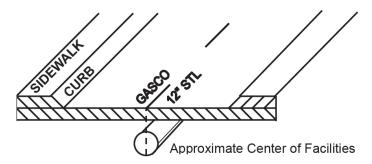
2) placing the marks over the approximate outside edges of the facility with a line connecting the two horizontal lines (in the form of an H) to indicate there is only one facility:
