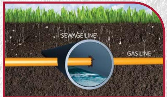
Plumbers typically use a mechanical rotary tool, or root cutter, to clear a sewer line. Clearing blockages with a mechanical rotary tool can damage a natural gas line that has been unknowingly bored through a sewer line. Natural gas can then migrate through the sewer line into a connected structure, including one without natural gas service. This migration creates the potential for a natural gas accumulation and possible deadly ignition.
